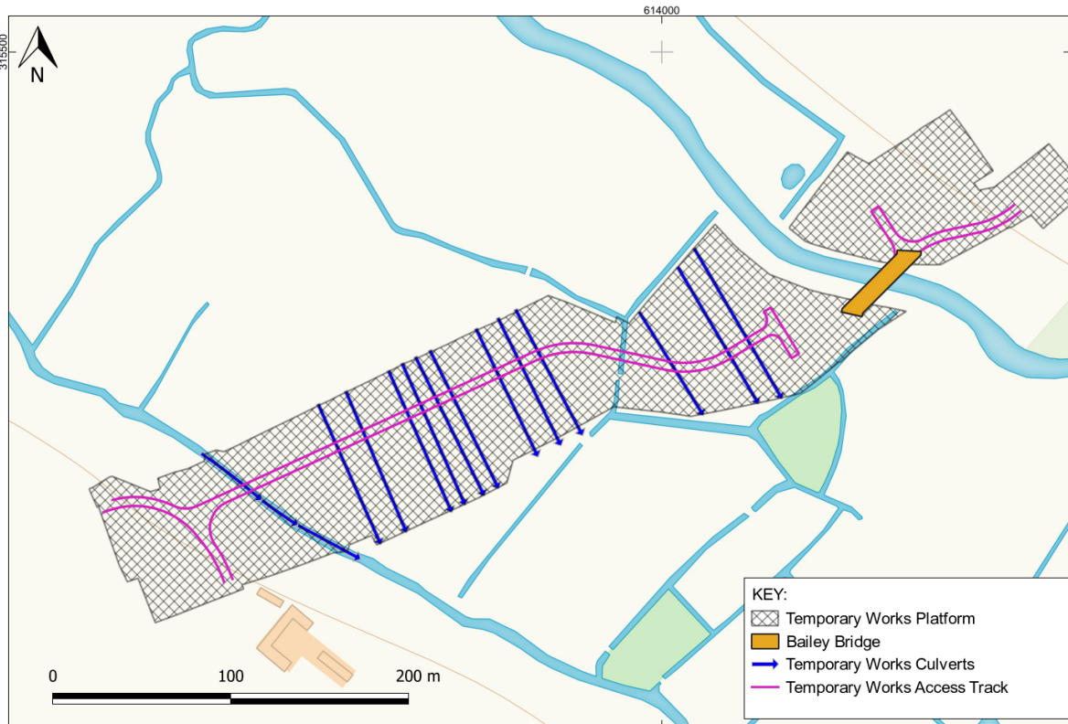
Figure 4-2 Details of the temporary works in the vicinity of the River Wensum
